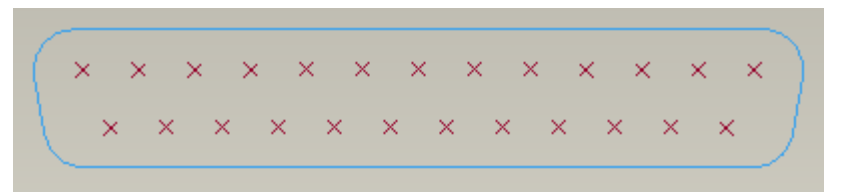
Skeleton Part Showing Pattern of Datum Points
