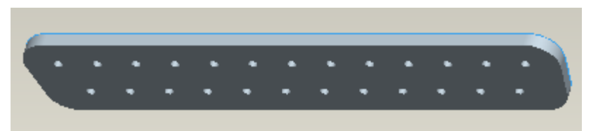
Component Referencing the Pattern in Skeleton
